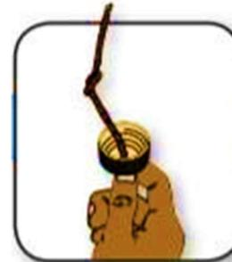
Tie a knot in the end of the rope, on the inside of the cap.
