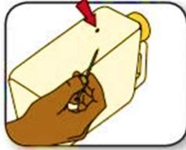
The tippy tap needs a hole for the water to pour out of. The hole should be on the side of the container across from the handle. The hole should be a finger length from the top of the container. Find the spot for the hole and make a mark there.
