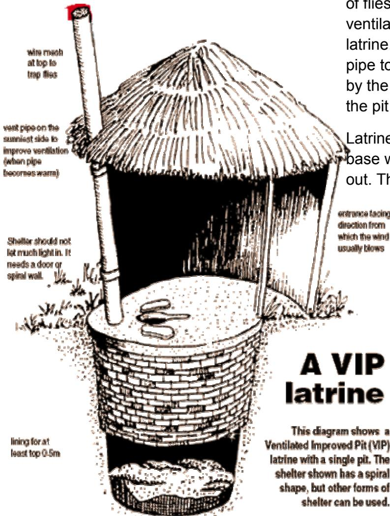
This diagram shows a Ventilated Improved Pit (VIP) latrine with a single pit. The shelter shown has a spiral shape, but other forms of shelter can be used.
